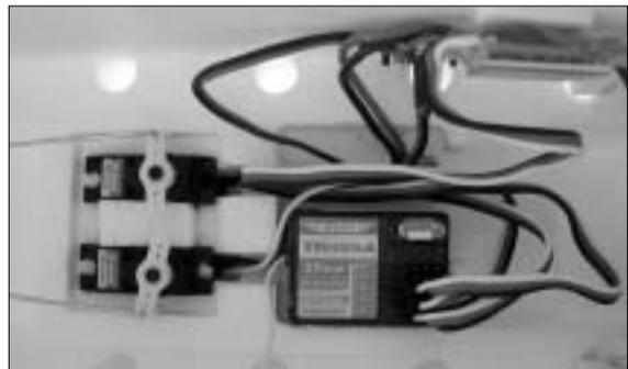
30. Connect all servo wires and controller wire. Normally the controller wire plug into the channel 3rd ( throttle). The Servo wire plug into channel 1(Aileron) and channel 2(Elevator).
