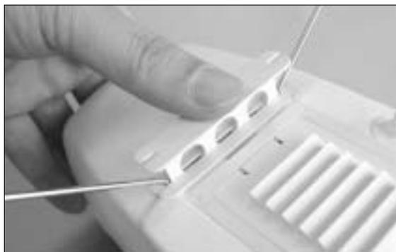
17. Insert the landing gear in the fuselage then "Push-N-Lock" the landing gear retainer.
