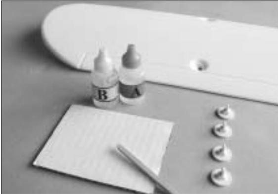
2. Mix the furnished 5-min Epoxy to glue the strut mount. Hint: Apply equal volume of cement in bottle A and B on a cardboard then fully mix them with a small stick. Note: This 5-min Epoxy allows working time is only 3 minutes after mixing.
