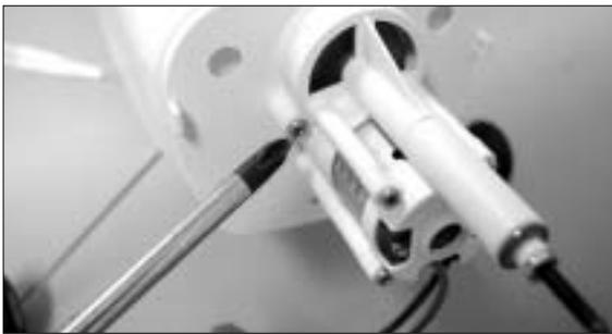
20. Secure the EDS with furnished two 3x20 self-tapping screw. Thread the Controller motor wire through the firewall from inside of fuselage then connect to the motor wire firmly. You may apply a piece of tape to prevent from it loose. Next thread the wire back to fuselage.
