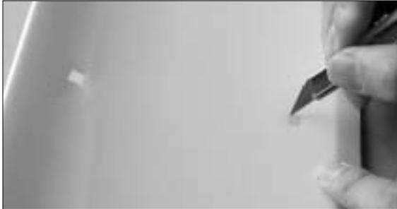
1. Carefully trim the strut mount hole in square then trail fit the strut mount in the hole. Make sure the strut mount is level with the wing surface.
