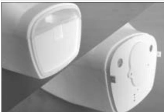
14. Trial fit the plastic firewall on the front of fuselage. Apply Epoxy at the rim of front fuselage then glue the firewall in place.
