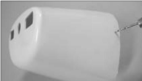
21. Drill 1/16" hole on the molded dot of the cowling.
