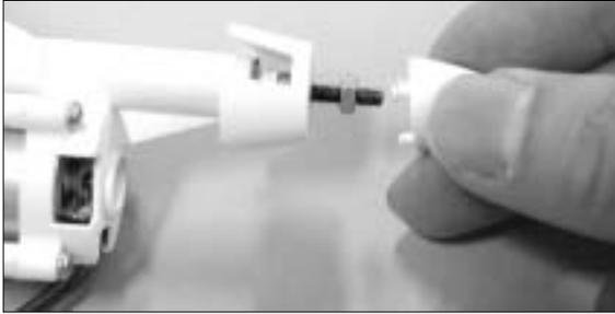
19. Locate the EDS (electric drive system) and remove the spinner and nuts. Note: Remove the nose cone by rotating it counter-clockwise about 1/4 turn.
