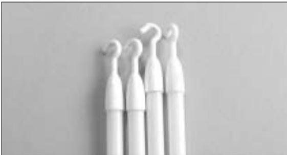
8. Locate the hooks and plastic tubs then glue the hooks onto one end of the tubs all the way in.
