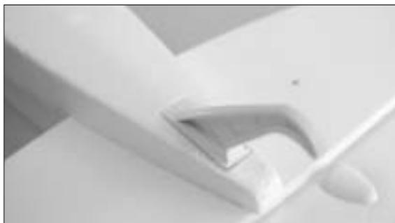
15. Epoxy the skid in place as shown.
