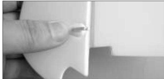
11. Locate the control horn and locking plate then "Push-N-Lock" the control horn in place as shown. Note: Do not push too hard but gently all the way in so the control horn contacts the surface of rudder at both sides and secured in place firmly.
