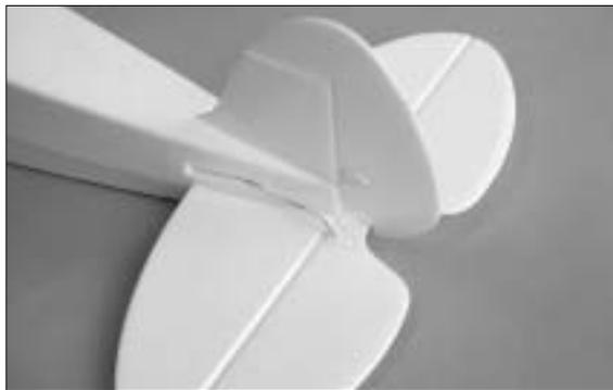
13. Trial fit the horizontal tail and vertical tail in the fuselage, epoxy the them in place when satisfied. Make sure they are perpendicular to each other.
