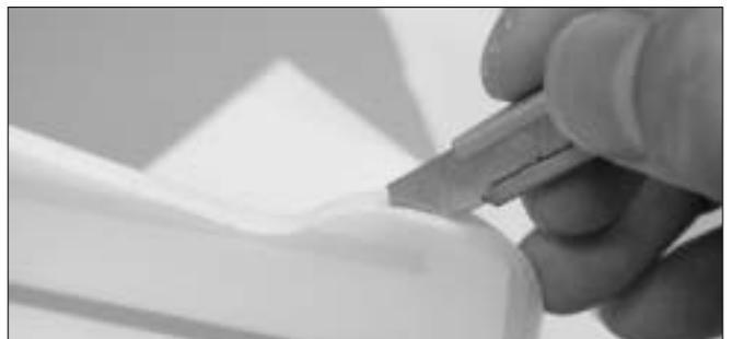
9. Locate the tail skid, next use hobby knife to cut a slot at the bottom of fuselage tail. Then insert the tail skid in place.
