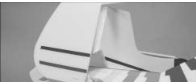
11. Use the furnished tape to tape the Rudder in place. Tape the left side first then the right side.
