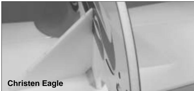
6. Use furnished square and make sure wing is perpendicular to the fuselage while gluing wing and fuselage together.
