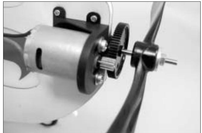
30. Locate M3 nut, put it in the propeller then thread the propeller on the drive shaft. Next attach propeller washer and another nut. Secure it firmly and make sure to leave at least 6mm drive shaft for rubber spinner.
