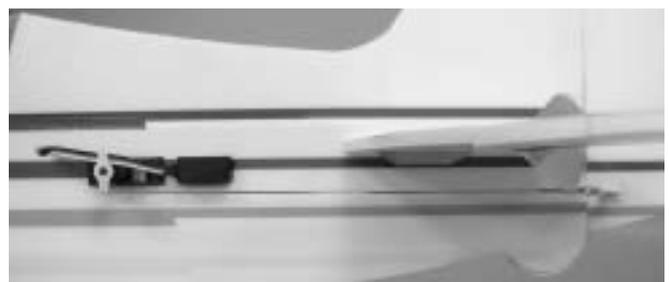
25. Install the elevator and rudder pushrods when servos are in neutral position and make sure rudder and elevator are even with the vertical fin and horizontal tail respectively.
