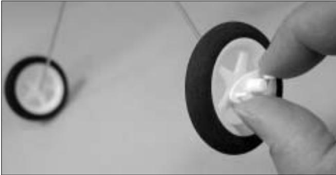
15. Install wheels by threading the wheel pant retainer in proper position.
