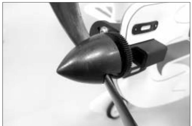
31. Install the rubber spinner on drive shaft properly and make sure it is not transformed.
