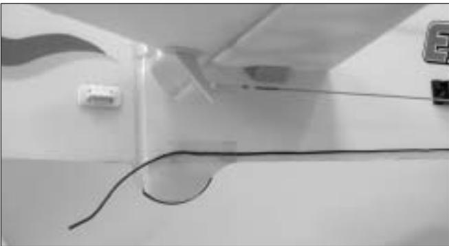
33. Route the antenna wire to the tail and tape it on fuselage.
