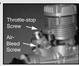
the airbleed screw about 1/2 turn. If the idling speeds up with the nose down, then stop the engine and open
