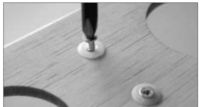
32. Locate the plastic washer and 3x20mm Wood Screw then secure the tail on the T-tail mount. Make sure the horizontal tail is perpendicular to the vertical tail and has same angle to the main wing if you see from the nose.
