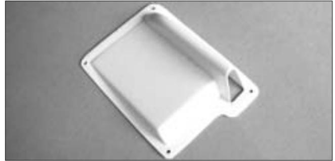
9. Locate the Hatch Cover and trim it along the molded line. Cut a hole as an exit for pushrod and drill holes at each corner with 1/16"(1.5mm) drill bit.
