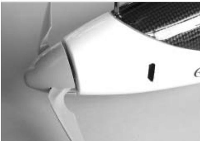
39. Make sure there is about 2~3mm(5/64"~1/8") gap between spinner backplate and fuselage.
