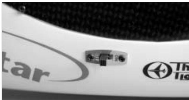
45. Use switch plate as a template, drill holes then install the switch as shown.
