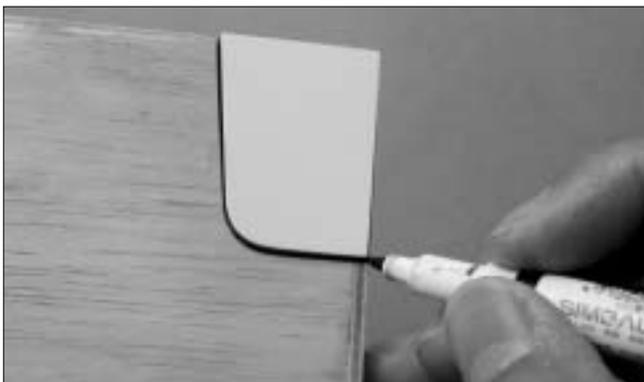
18. Locate the wing protectors, place the wing protector where is even with the edges. Make marks along the wing protector on the wing.
