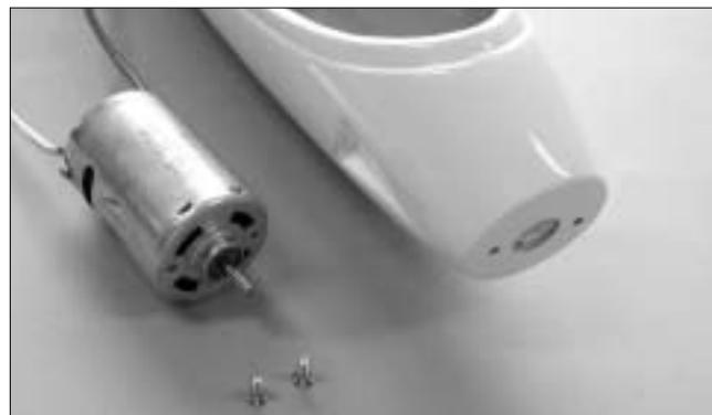
37. Locate the motor, and 3x8mm countersunk screws. Secure the motor in the fuselage.
