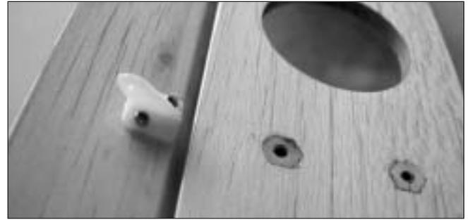
30. Drill 2mm holes and install the control horn on the tail, note it has to be in line with the tail mounting holes and the control horn is even with the elevator leading edge.
