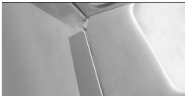
36. Locate the CA hinges then insert the CA hinges in the slots of the vertical tail then glue the rudder and CA hinge in place with thin CA.
