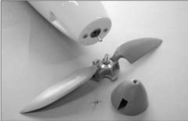
38. Locate the prop, spinner and screws as shown. Assemble the folding prop first. Make sure the two blades move freely. Insert the drive nut to the backplate then the drive shaft. The hole of drive nut is tapered to accommodate the drive shaft. Secure the whole set onto motor shaft with the nut. Do not over-tighten the nut as it might break the aluminum drive shaft but make sure it will not spin out when it in high rotation.
