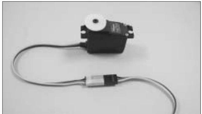
5. Connect the extension wire and tape the connector to prevent from disconnecting during flight.
