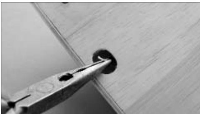
8. Pull the string out from the hole slowly, using needle-nose pliers or tweezers.
