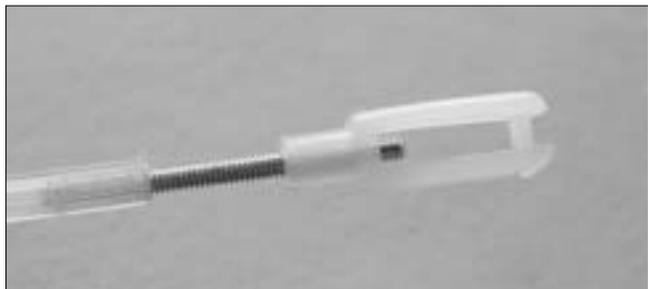
33. Locate the short/ long threaded end, clevis and plastic tube. Thread the long threaded end to plastic tube first about 1/4" (6mm) in length then insert the plastic tube through the guide tube from the bulkhead end. Get the plastic tube at the rear of T-Tail mount then install the short threaded end and clevis.
