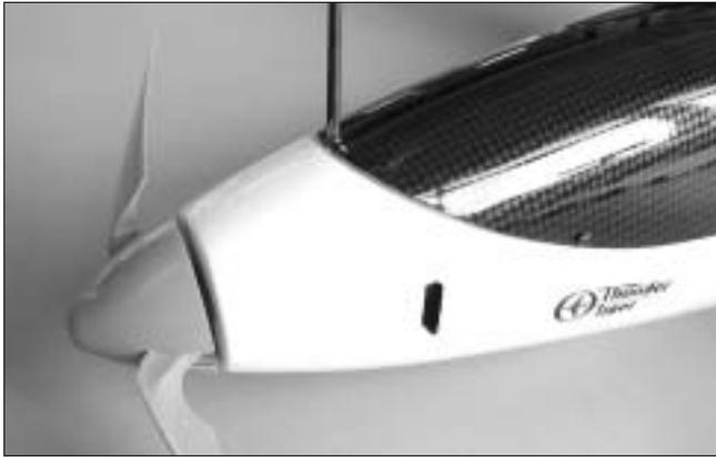
47. With the canopy in place on the fuselage, drill 5 holes with 1/16" (1.5mm) bit. One in the front of canopy, two at both sides of the canopy. Next secure the canopy with 2x5mm wood screws.
