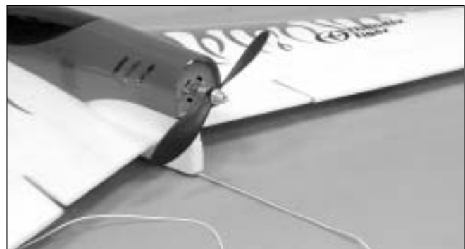
25. Route the antenna through the tube as shown.
