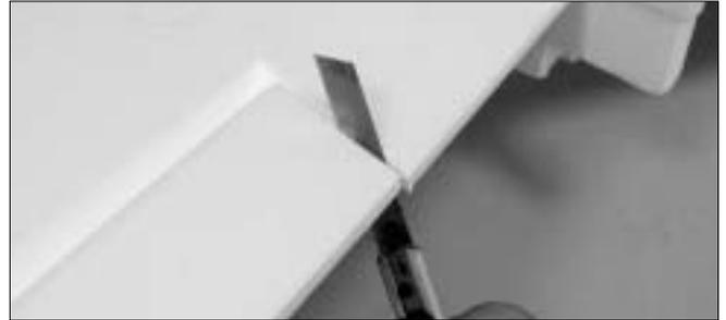
1. Cut trailing edge for aileron control surface along with the molded line with hobby knife. Note: do not cut hinge line.
