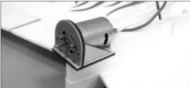
13. Epoxy the motor mount assembly at the tail. Make sure the motor mount is all the way in the fuselage and secured firmly after it is cured.
