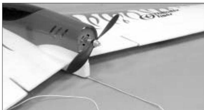
25. Route the antenna through the tube as shown.
