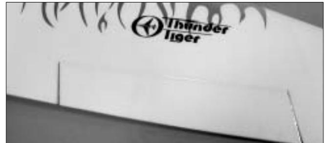
3. Apply decal on the wing. Attached to the leading edge first then carefully apply decal on the wing surface to the trailing edge. Note: Do not cut away the transparent area, as it will cover the aileron area.
