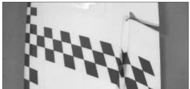
4. Locate the flag strip then apply it at the bottom wing surface. Note: Do not cut away the decal at the hinge line. This decal will help holding the aileron in place.
