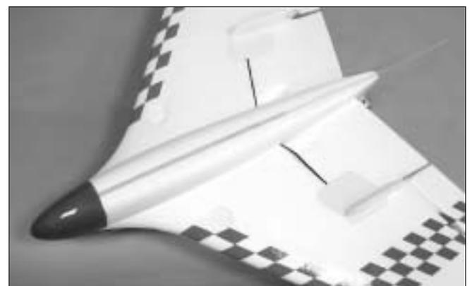
18. Epoxy the wood skid and antenna tube at the bottom fuselage as shown.
