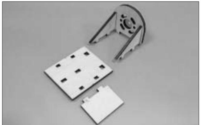
11. CA or epoxy the fiberglass and plywood firewall together then glue the plywood part D on firewall.
