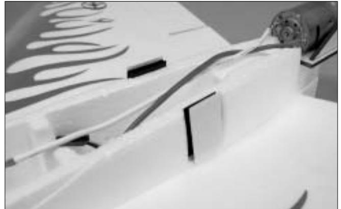
16. Locate Velcro and cut it into two pieces. Attach Velcro on the two sides of fuselage.
