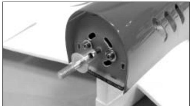
24. Locate the drive shaft then secure the drive shaft on motor with the furnished setscrew and hex wrench. Next secure the propeller with the prop nut. Note: the drive shaft and prop nut are in opposite thread. Thread the prop nut counter clock-wise.
