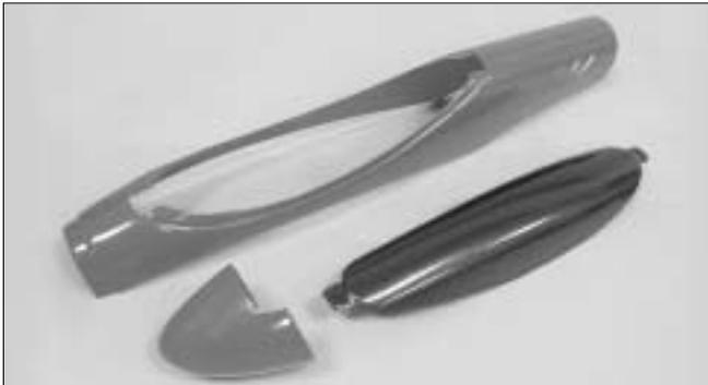
14. Trim deck, canopy and nose cone along with the molded line as well as the cooling slots at the tail of deck. You need to trim the canopy tabs and deck to get a good fit when canopy is installed on the deck.
