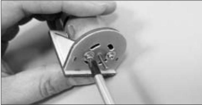
12. Next glue the part A and B to complete whole motor mount. Secure motor with M2.6x8 screws and washers.
