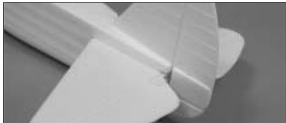
21. Epoxy the vertical fin in place and make sure it is perpendicular to the horizontal tail. Trim the trailing edge of the rudder and fuselage tail if necessary.
