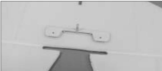
17. Cut a slot at the hinge line for installation of elevator joiner.
