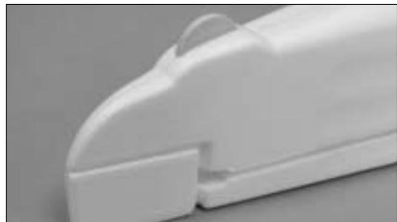
13. Locate the round plywood and glue it in tail bottom slot as a tail skid/wheel.
