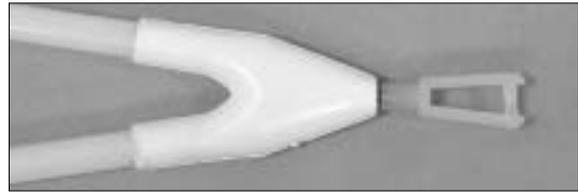
50. Assemble the wing strut joiner as shown, you will need to thread the threaded rod to the wing strut joiner first then thread the clevis. A needle nose pliers will help thread the rod. Epoxy the two plastic tubes to the joiner; one is long and the other is short.
