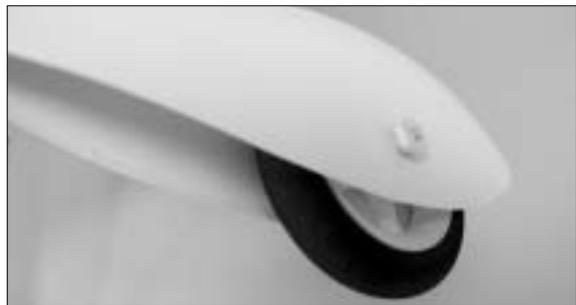
29. Install the wheel pant and wheel on landing gear next thread the plastic nut. Make sure wheel rotates freely.
