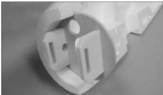
4. Trial fit the firewall assembly in right fuselage half,
