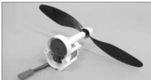
31. Locate the EDS( electric drive system) and remove the spinner and nuts. Note: remove the nose cone by rotating it counter-clockwise about 1/4 turn.
