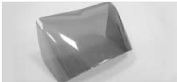
44. Locate the canopy and trim it along with the molded line as shown.
