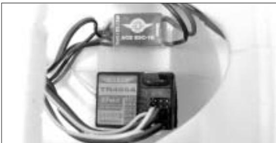
41. Use double sided tape to fix the ESC and
