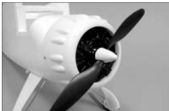
37. Install the propeller and spinner. It is necessary to secure the propeller firmly by a 3mm nut. Always take great care on the motor and swinging propeller as it is dangerous and may cause serious injury, if you are a beginner we recommend you read the manual of radio and speed controller thoroughly to understand how to set up and control the motor.
