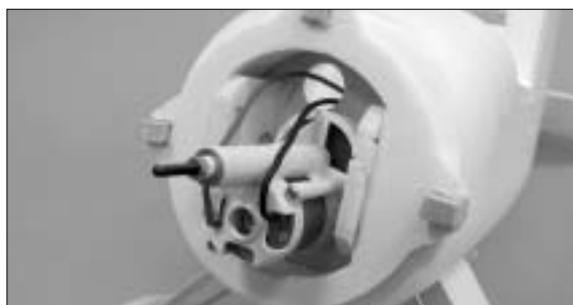
32. Install the power drive unit in place with two 3x20 wood screws. Thread the motor wire through the firewall.
