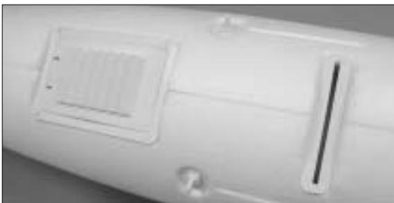
10. Locate the battery box and landing gear mount next epoxy them in place as shown.
