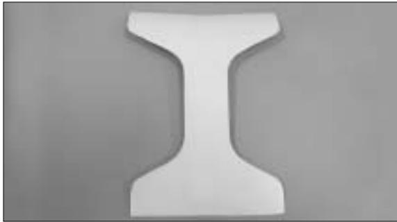
46. Locate the wing center cover then trim it along the molded line as shown.
