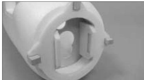
12. Glue the cowling mount A on mounts B and C. Locate three balsa wood blocks then glue them in place as shown.
