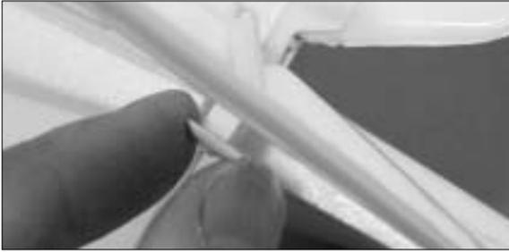
23. Install the rudder control horn. Make sure the control horn is installed properly before you press in the locking plate and do not over press the locking plate.
