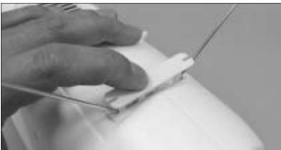
26. Insert the landing gear in the landing gear mount then press the retainer all the way in to secure the landing gear in place. When pressing make sure to support from the inside of fuselage.
