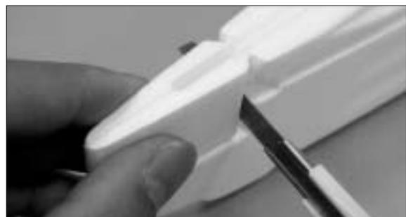
14. Carefully cut off the tail, this portion will be glued on rudder later. Sand the cut area if necessary.
