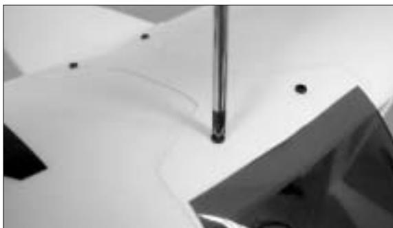
49. Drill 2mm mounting holes on the molded dots. Secure the main wing with two 3x30mm (front wing bolt) and two 3x25mm (rear wing bolt) wood screws.
