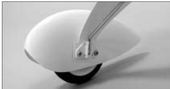
30. Secure the wheel pant with two 2x5mm wood screws as shown. Do the same procedure on the other wheel.
