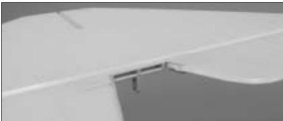
18. Trial fit the joiner in place next apply epoxy and glue it firmly in place. It will be easier to bend two elevators then slide the joiner on the elevator.
