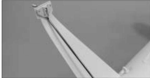
28. Install the wheel pant retainer then the landing gear fairing. Insert the fairing root into the slot you cut in the prior step. The fairing is for scale look it may effect the performance. For better stability, you may trim the fairing narrower.
